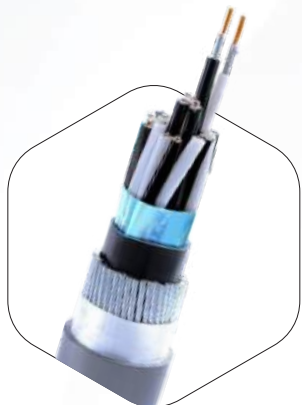
Overall Shielded, Armoured, Fire resistant, Instrumentation Cables 300/500V - 600/1000V BS EN 50288-7, Generally to IEC 60502-1, IEC 60331-21, BS 6387 (CWZ), IEC 60332-1-2, IEC 60332-3-22 (CAT A), IEC 60332-3-24 (CAT C)
