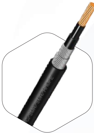
Copper Conductor, HMWPE Insulated, Double Layer of Galvanized Steel Wire Armor & HMWPE Outer Sheathed, 600/1000V
