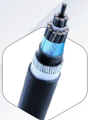
Overall Shielded, Armored, Flame Retardant, Instrumentation Cables 300/500V - 600/1000V BS EN 50288-7, Generally to IEC 60502-1, IEC 60332-1-2, IEC 60332-3-22 (CAT A), IEC 60332-3-24 (CAT C)
