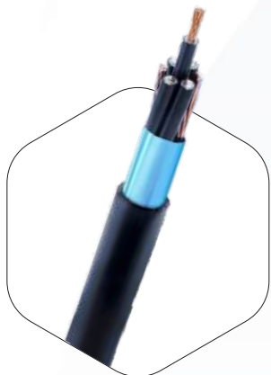
Overall Shielded, Un-Armoured, Flame Retardant, Instrumentation Cables 300/500V - 600/1000V BS EN 50288-7, Generally to IEC 60502-1, IEC 60332-1-2, IEC 60332-3-22 (CAT A), IEC 60332-3-24 (CAT C)
